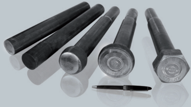
Picture 4: JUMBOTECH® Production Process, Hexagon Stud M36
